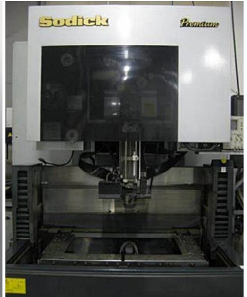
Wire cutting machine[AQ537L] (Sodick)
