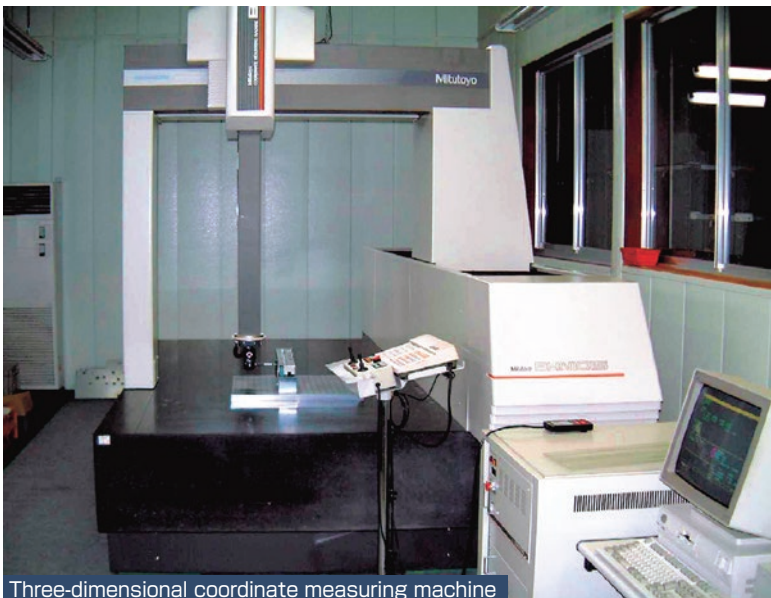
High-sensitivity 3D CNC coordinate measuring machines fitted with non-contact sensors, suitable for use with computer aided verification
