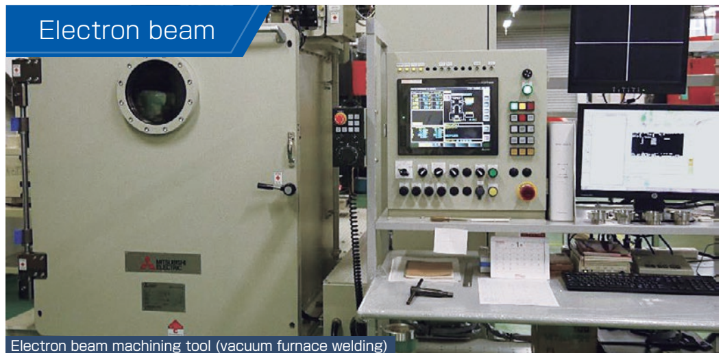
Electron beam machining tool (vacuum furnace welding)
