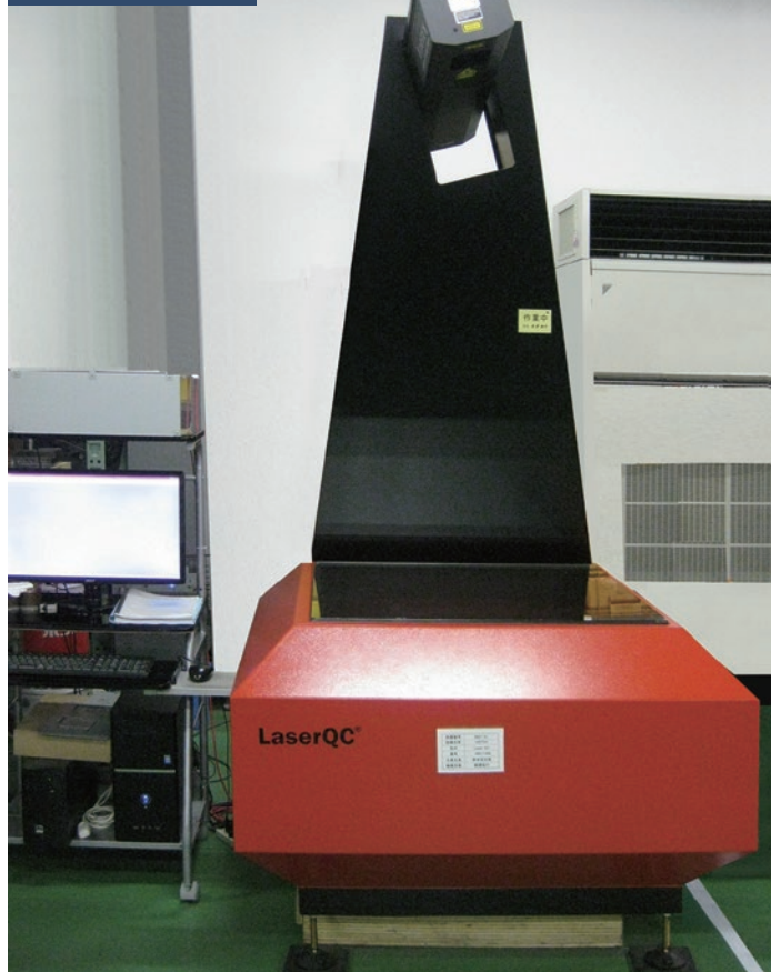
Virtek infrared measuring instrument
