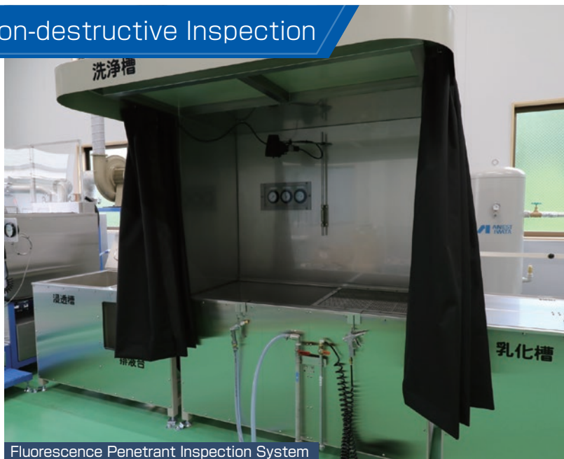
Fluorescence Penetrant Inspection System
